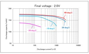
\* Nominal capacity indicates duration until the voltage drops to 2.0 V when discharged at a nominal discharge current at 20 deg. C.
