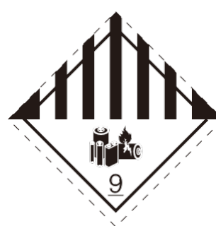
Lithium battery hazardous label
